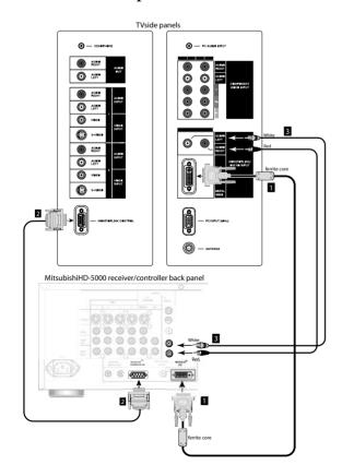
Figure 14. Connecting MonitorLink
